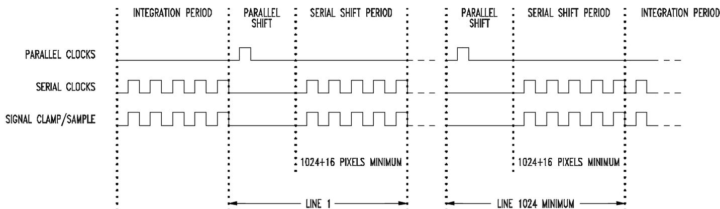
FIGURE 4 Typical full-frame readout
