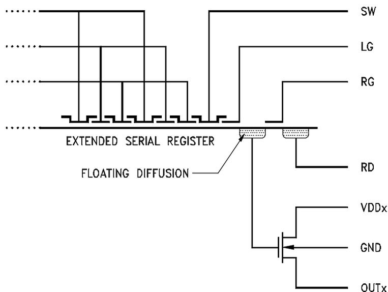
FIGURE 1 Output Structure
