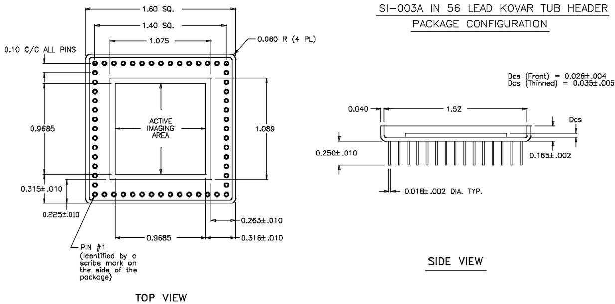
FIGURE 6 SI-003A package configuration
