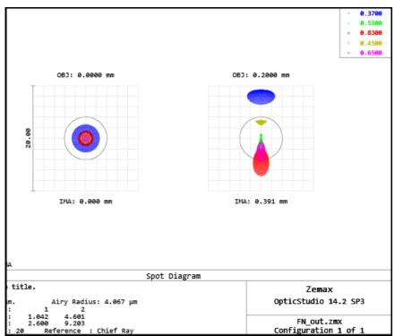
Illustration 6: Spot diagram of the FN output system
