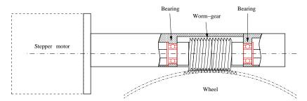
Figure 1: Schematic of Worm-wheel showing problem bearings
