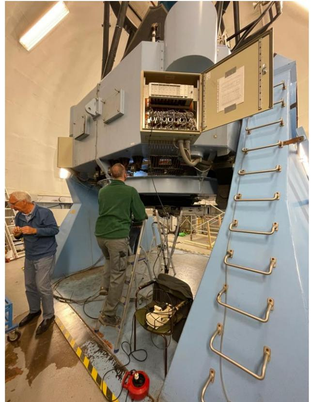
Figure 4: Roughing pump connected bellow o1b1.
