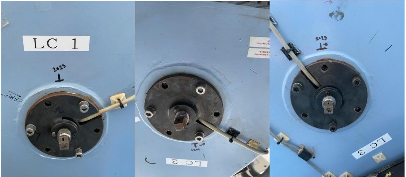
Figure 7: Photographs of each load cell as adjusted and marked in 2023. The T-bar measured LC heights are marked with the upside-down T-symbols on the mirror cell. Radial line indicates the direction normal to the marked face of the adjustment screw. For example, LC1 is as measured with the T-bar, and LC2 close to 180° rotation towards the direction indicated by arrow.
