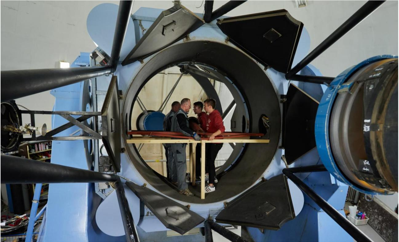
Figure 5: T-bar coming out of the telescope after contact measurement of M1 with a help of a wooden jig on which it can be rested.
